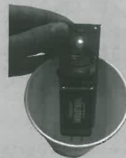
611-2263 Blinking LED Meter When both electrodes are submerged in a solution, our little meter struts its stuff. It remains off if the solution is non-conductive but glows dully in a weak one. When encountering a strong conductor, it blinks brightly.
