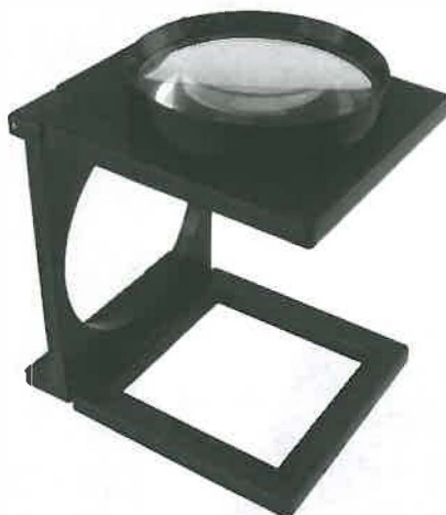
631-7010 Foldable Magnifier This upright plastic magnifier locks into place and has an in/ cm grid for reference. Large, 4" (10cm) diameter plastic lens. 2X magnification.
